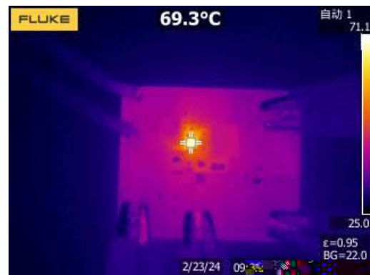
Figure 29. Thermal, 24VIN, 5VOUT, 0.8A
