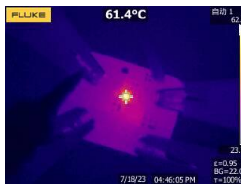
Figure 20. Thermal, V_{IN}=5V , V_{OUT}=1.2V , I_{LOAD}=3A
