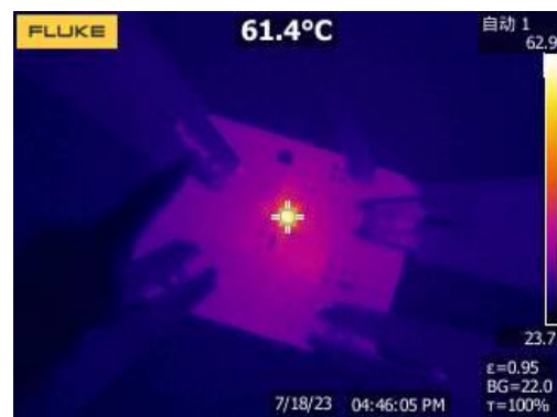
Figure 20. Thermal, V_{IN}=5V , V_{OUT}=1.2V , I_{LOAD}=3A
